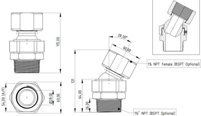
Example: GW 1<sup>1</sup>/<sub>2</sub>" Swivel Adapter fitted with GW Thermoshield 883B nozzle
