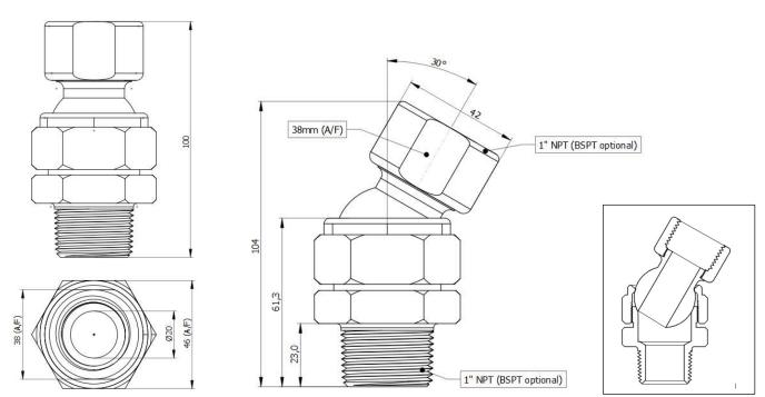
Example: GW 1" Swivel Adapter fitted with GW Fyrhed WF nozzle
